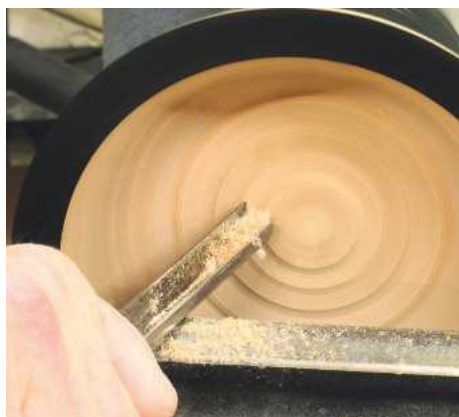
▲ Pic.2 The heel of the tool is ground off by resting the tool on the toolrest with the flute pointing towards you. This will stop you rubbing too much bevel on the workpiece and over-compressing the timber
